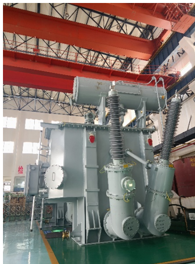
SFPZ11-16000/35 Mobile Transformer Russia
